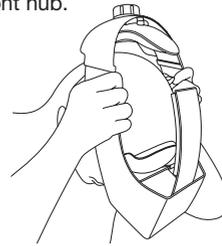
2. Turn the size adjustment knob counter-clockwise to make the size bigger.
