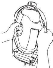
6. Turn the size adjustment knob to lock the main unit into position.
