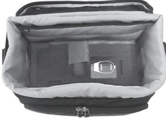
2. Place the main unit on the calibration kit, and firmly close the lid of the storage bag.
